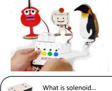
Solenoid is a electromagnet that pulling the plunger when energized.
