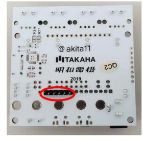
Connect a power such as a mobile battery to this board.
