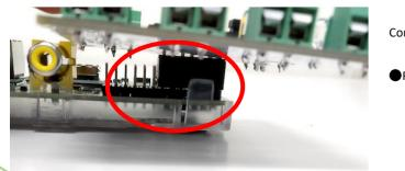
Connect a power such as a mobile battery to this board.
