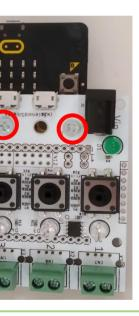
micro:bit IO pin 0-2 react to solenoid #1-#3 solenoid #4 is uncontrolled •Set IO pins 1 and 2 as output -1 (HIGH) = ON -0 (LOW) = OFF
